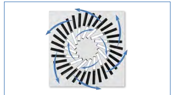
Outer air control blades set to external swirl, inner blades set to internal swirl
