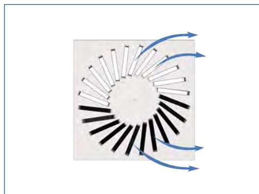
Setting of the air control blades
