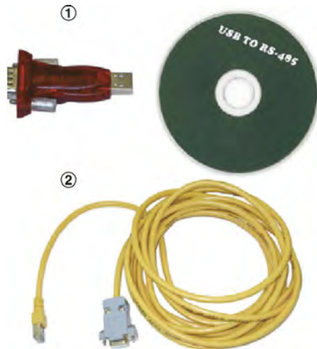
Fig. 17: Adapter and connecting cable
