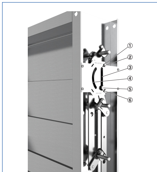
Schematic illustration of the quadrant stay and limit switch (steel multileaf dampers)
