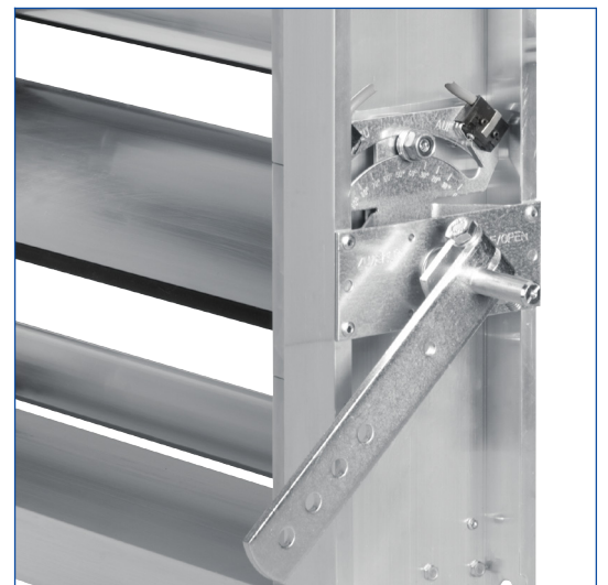
The quadrant stay is situated on the first blade from the top (dampers with up to three blades) or on the third blade from the top (dampers with at least four blades)
