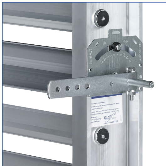
The quadrant stay is situated on the first blade from the top (dampers with up to three blades) or on the third blade from the top (dampers with at least four blades)
